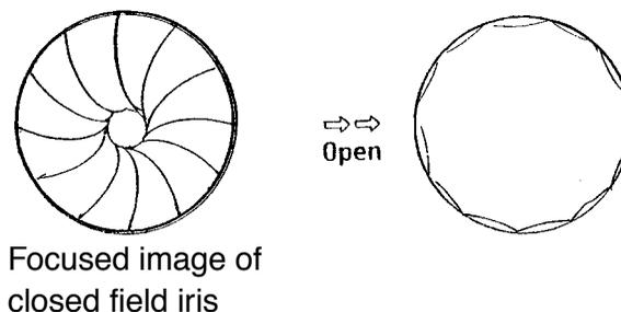
(7) Removing one of the eyepieces, observe the disc of light coming from the back of the objective in use. Close down the aperture iris⑧, using the lever on the substage condenser, until only about 70%-80% of the disc of light observed remains visible. (Note that the microscope is now set up for use with the 10X objective. Similar adjustments to those mentioned above should be made when using any of the objectives required.)
