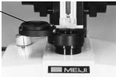
The substage polarizer⑬ is fully rotatable with a swing-out, click-in mount. When the polarizer is swung out, the light is not polarized.
